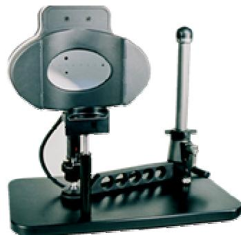
The pattern stimulator has been designed to produce standard ISCEV patterns on a monitor for VEP and ERG tests.
