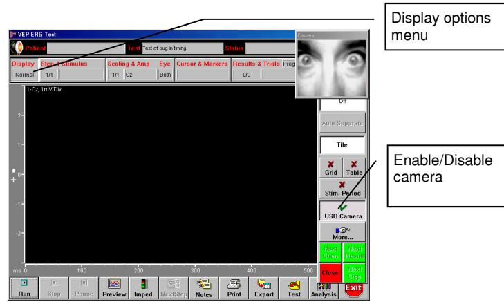
**Note:** The frame update timing of the image displayed on the Espion screen is refresh limited by many factors to no more than a few Hertz which is normally too slow to catch patient blinks. For real-time display, you must attach an external monitor.
