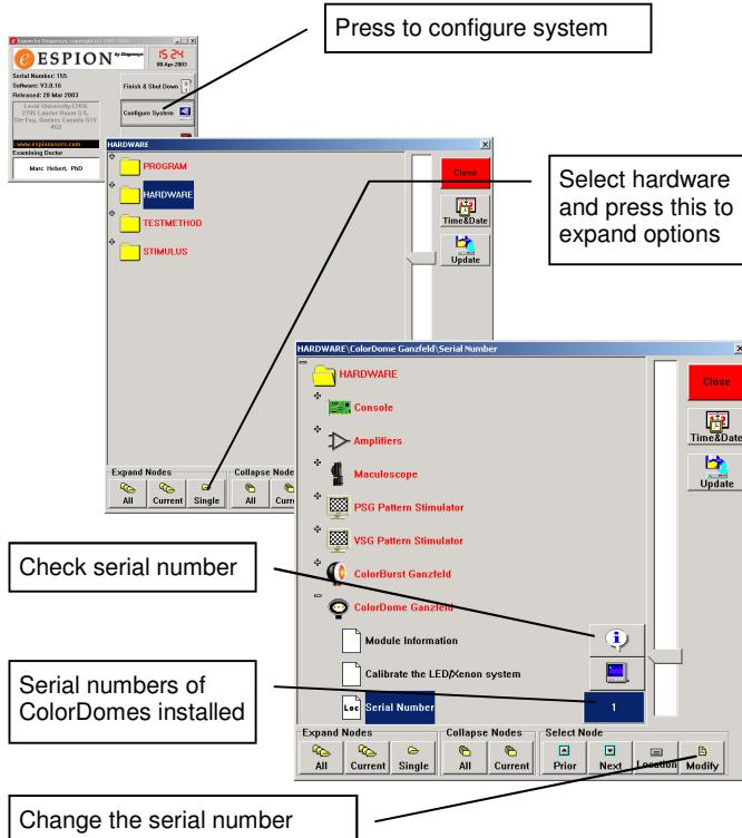
To change the serial number, select the serial number parameter in the ColorDome hardware section and press the modify button at the bottom of the screen. If you have two ColorDomes, then enter both serial numbers. Finally exit the menu by pressing the red Close button in the top right. To check that the calibration file has been correctly read, re-enter the configure system menu and press the "l" information button. This will produce the information menu which
