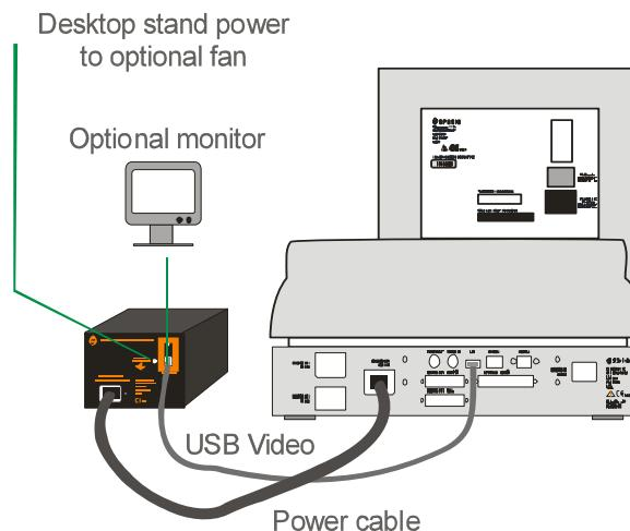
Rear connections from the power box to the PowerBlok include the mains power cord (Note: this must NOT be connected directly to a mains outlet as this compromises the ColorDome electrical isolation) and the USB video cable. The
