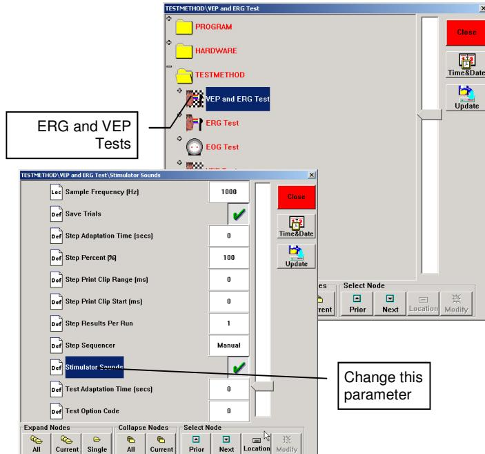
This audible output can be enabled and disabled from the "Configure System" menu, by changing the "Stimulator Sounds" parameter of the relevant "Testmethod" module.
