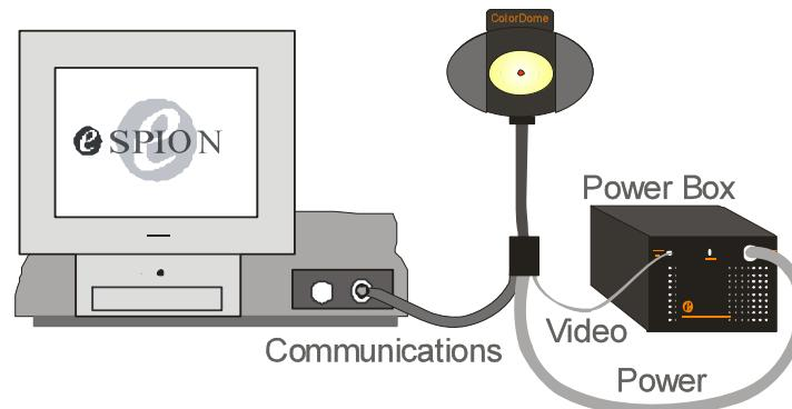
The three connections carry the camera video, low voltage power cables and communications from the Espion console.
